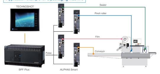
The film, conveyor, pinch roller and sealer operate synchronously with the operational pattern being automatically calculated from the length of the cut.
